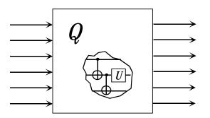
The 2-qubit XOR or "controlled-NOT" gate flips its 2nd input if its first input is 1, otherwise does nothing.
