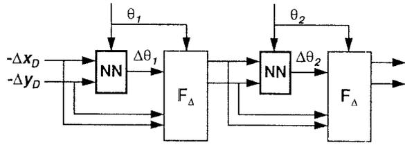
Figure 9: Incremental Back Propagation Through Links - neural network and link equations sequence
