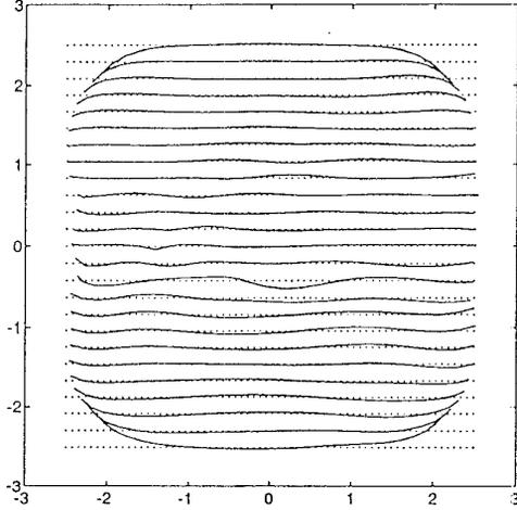
Figure 4: End-effector trajectories (solid lines) of a 3-link robot arm, commanded to follow straight lines (dotted)
