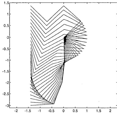
Figure 12: Incremental Back Propagation Through Links - 4-link robot arm
