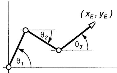
Figure 6: A planar serial manipulator with angles defined relatively to a base line
