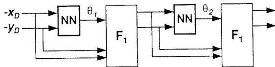
Figure 8: Back Propagation Through Links - controller structure
