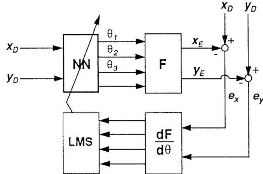
Figure 3: Training a “one step” controller, using the Jacobian matrix of the forward kinematics equations
