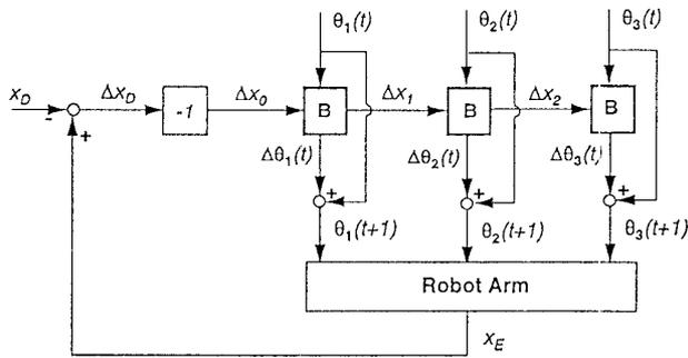
Figure 10: Incremental Back Propagation Through Links - closed loop controller structure
