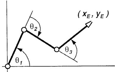
Figure 1: A planar serial manipulator
