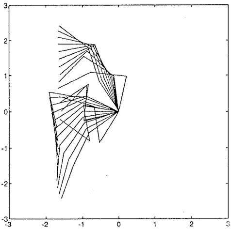
Figure 5: 3-link robot arm following a straight line
