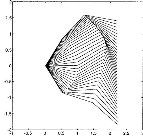
Figure 11: Incremental Back Propagation Through Links - 3-link robot arm
