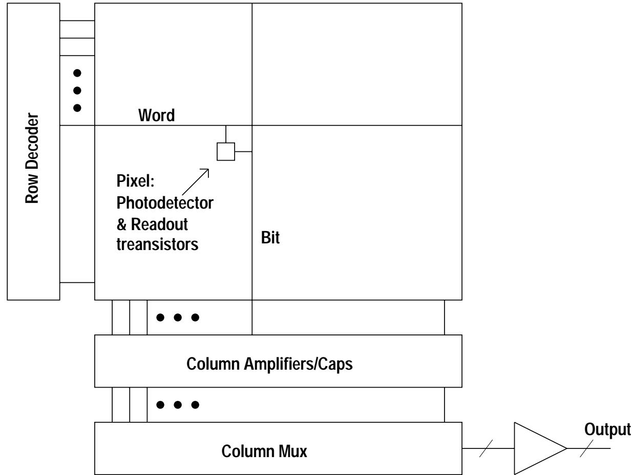
Most popular type called Active Pixel Sensor (APS), pixel has photodiode and 3 transistors
