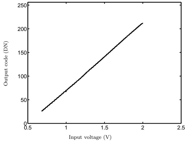
**Figure 6.** Measured ADC transfer curve.
