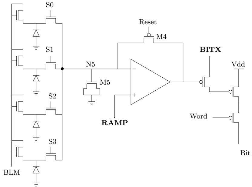
**Figure 2.** A  $2 \times 2$  pixel block sharing one ADC.
