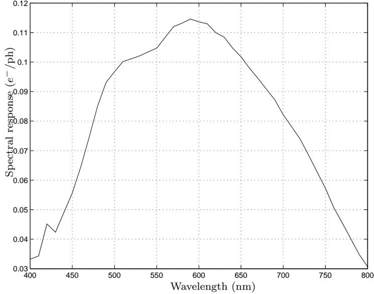
**Figure 7.** Measured average spectral response of the imager.
